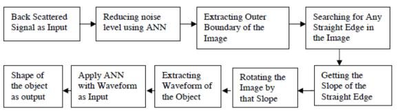
Fig 6. Block diagram of the system recognizing the shape of the buried object when orientation effect has neutralized.
