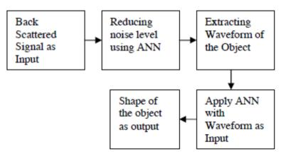
Fig 4. Block diagram of the system for recognizing the shape of the metallic shallow buried object without consideration of orientation effect.
