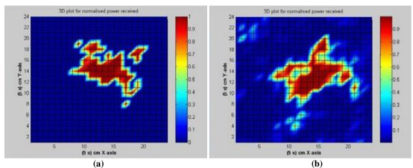
Fig 7. (a) Enhanced image obtained without rotation, (b) Enhanced image obtained after rotation.
